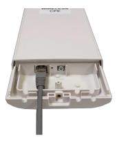
3. Slide the cover back to seal the bottom of the ZAC-1023.
