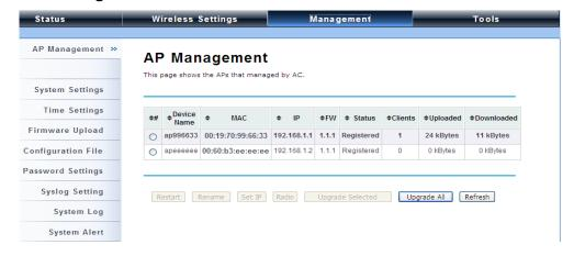
The configured AP in Virtual AC + Thin AP mode is highlighted in bold on the list. By selecting it and hitting the **Radio** button, you can configure the **channel bandwidth**, **channel antenna**, and **output power**.
