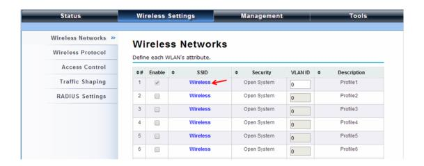
The ZAC-1023 will allow you to configure up to 8 virtual networks and encryption levels.
