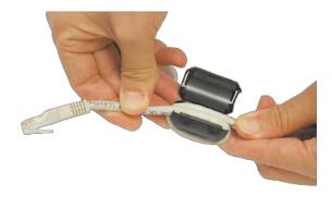
4. Close the core and snap the assembly back together.
