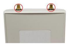
Connect the included external antennas to the SMA-RP connectors on top of the 1. CPE.
