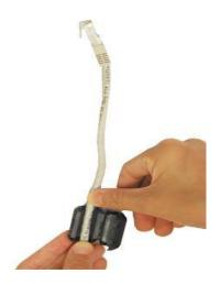
3. Loop the cable around and through the core. This may be required in circumstances with severe interference.
