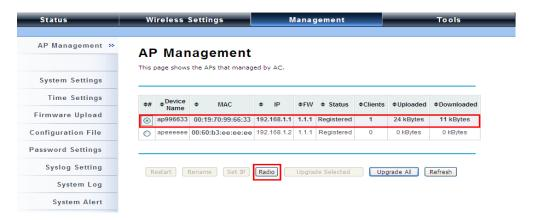
AP Management also allows you to reboot the managed AP, change its IP address, and perform firmware upgrades.
