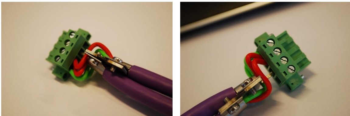
Fig. 26 - Use the Dual Ground Clip to connect two PROFIBUS cables in one screw terminal
