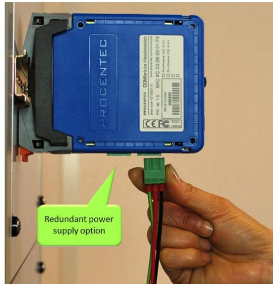
Powering the Head Station
