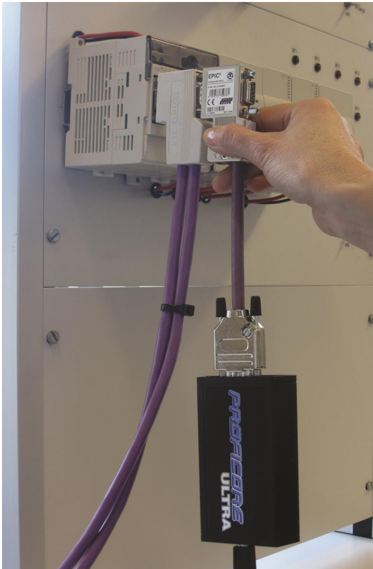
Fig. 10 - Attaching the ProfiCore to a DP installation
