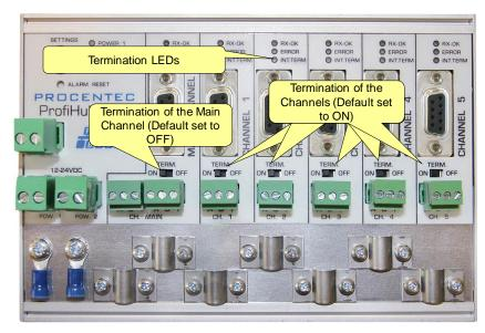
Fig. 15 - Termination Switches
