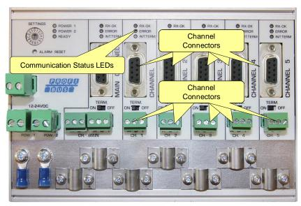
Fig. 14 - PROFIBUS DP spur connectors
