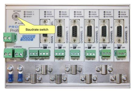
Fig. 16 - Baudrate speed switch
