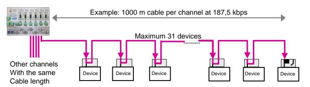
Fig. 6 - Cable lengths for PROFIBUS DP
