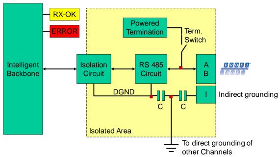
Fig. 5 - Channel structure
