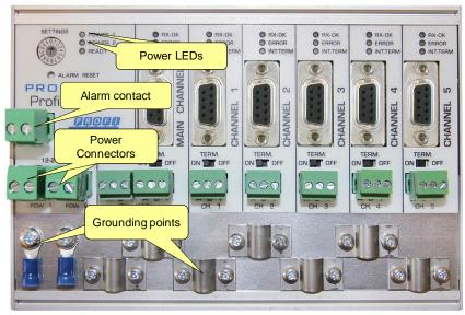
lFig. 10 - Power connectors and LEDs
