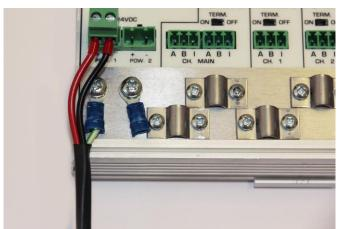
Fig. 12 - Connection to Ground Rail
