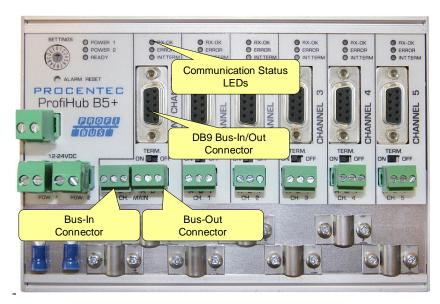
Fig. 13 - PROFIBUS DP backbone connection
