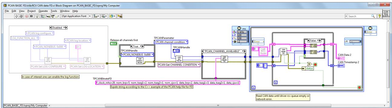
The disabled code segment is followed by the initialisation of the TPCANHandle (channel) and the hardware initialisation. Here is the biggest difference between CAN 2.0B and FD. FD is initialised by a string and not by API VIs.
